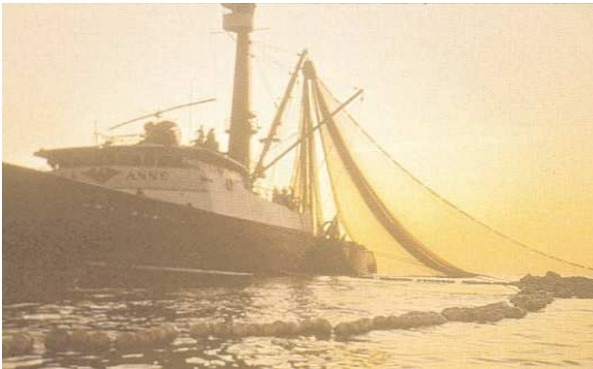
An industrial fishing vessel picking up a big pelagic drifting net, nowadays forbidden. On the top of the vessel is visible an helicopter employed for the big pelagics aggregates sighting.
